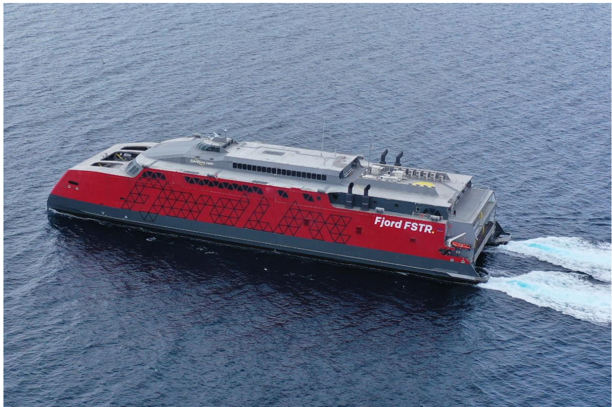
Fjord Line’s FSTR (Austal Hull 419) is a 109 metre high speed vehicle-passenger ferry, designed by Austal Australia and constructed by Austal Philippines (Image: Austal Philippines)
