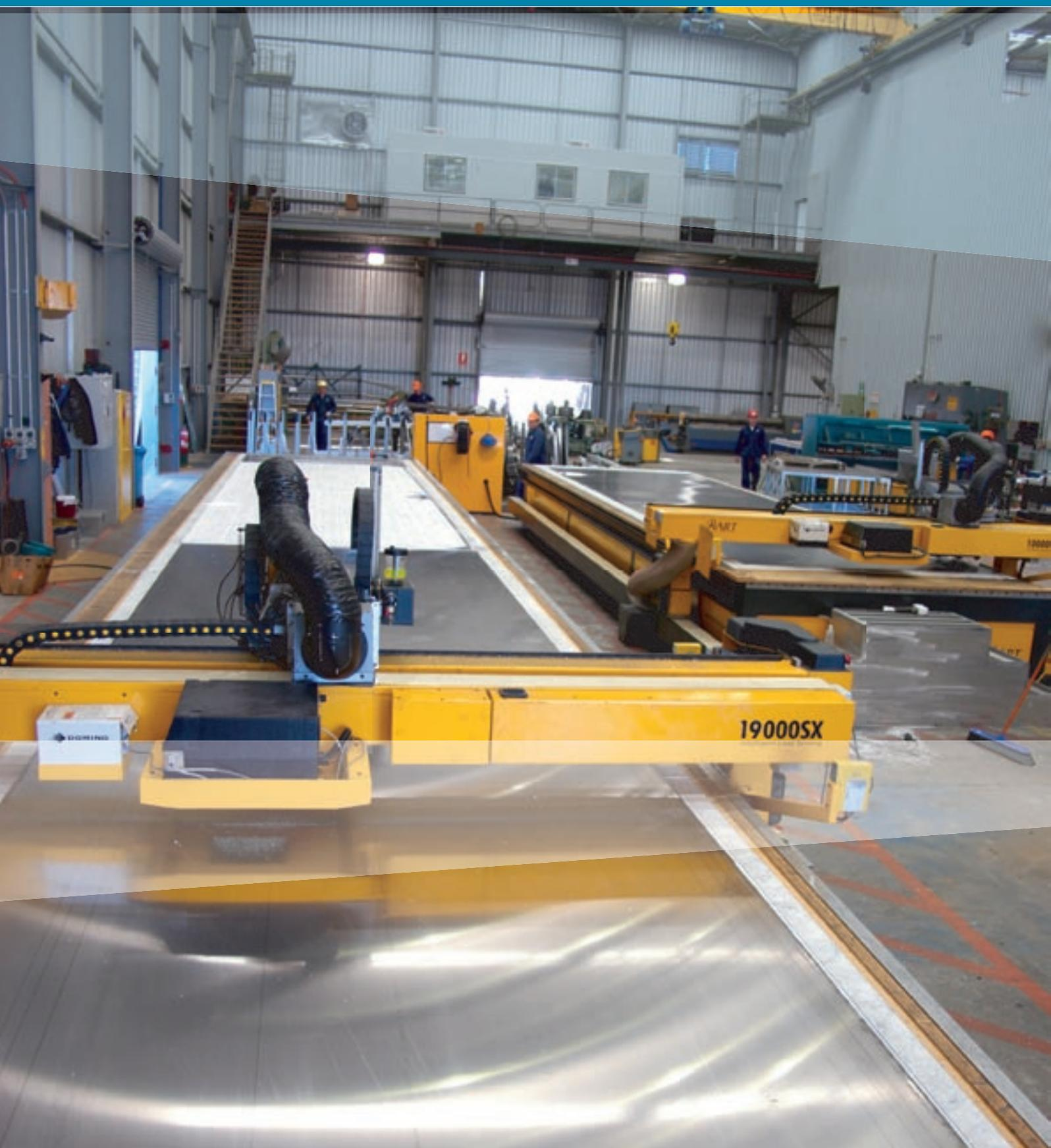
▲ The introduction of large routers in Austal's Australian and USA shipyards allows aluminium plate to be cut into precise pieces
