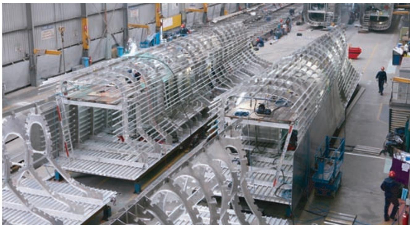
▲ Precise modules under construction prior to being attached to the main vessel
