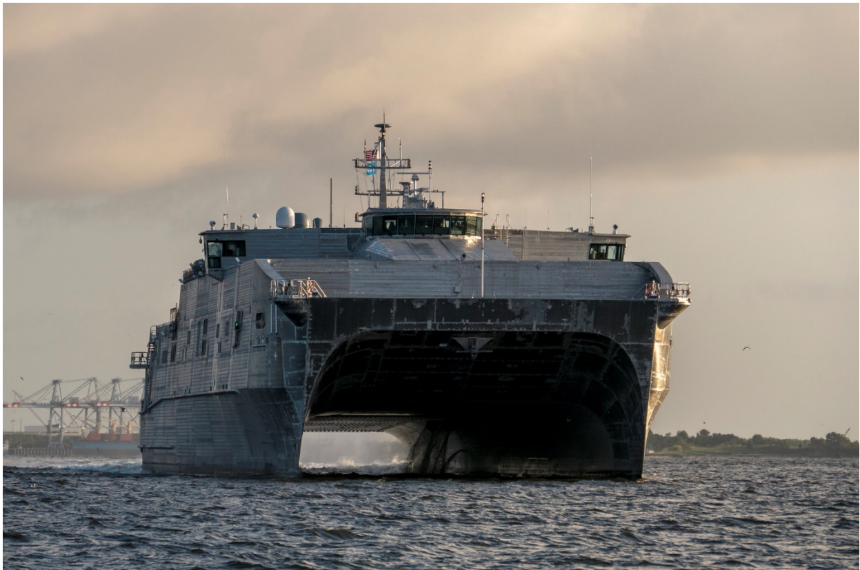
USNS Puerto Rico (EPF11) was the first EPF to perform and successfully complete integrated sea trials – combining builder's trials and acceptance trials into one at-sea event. (Image: Austal USA)
