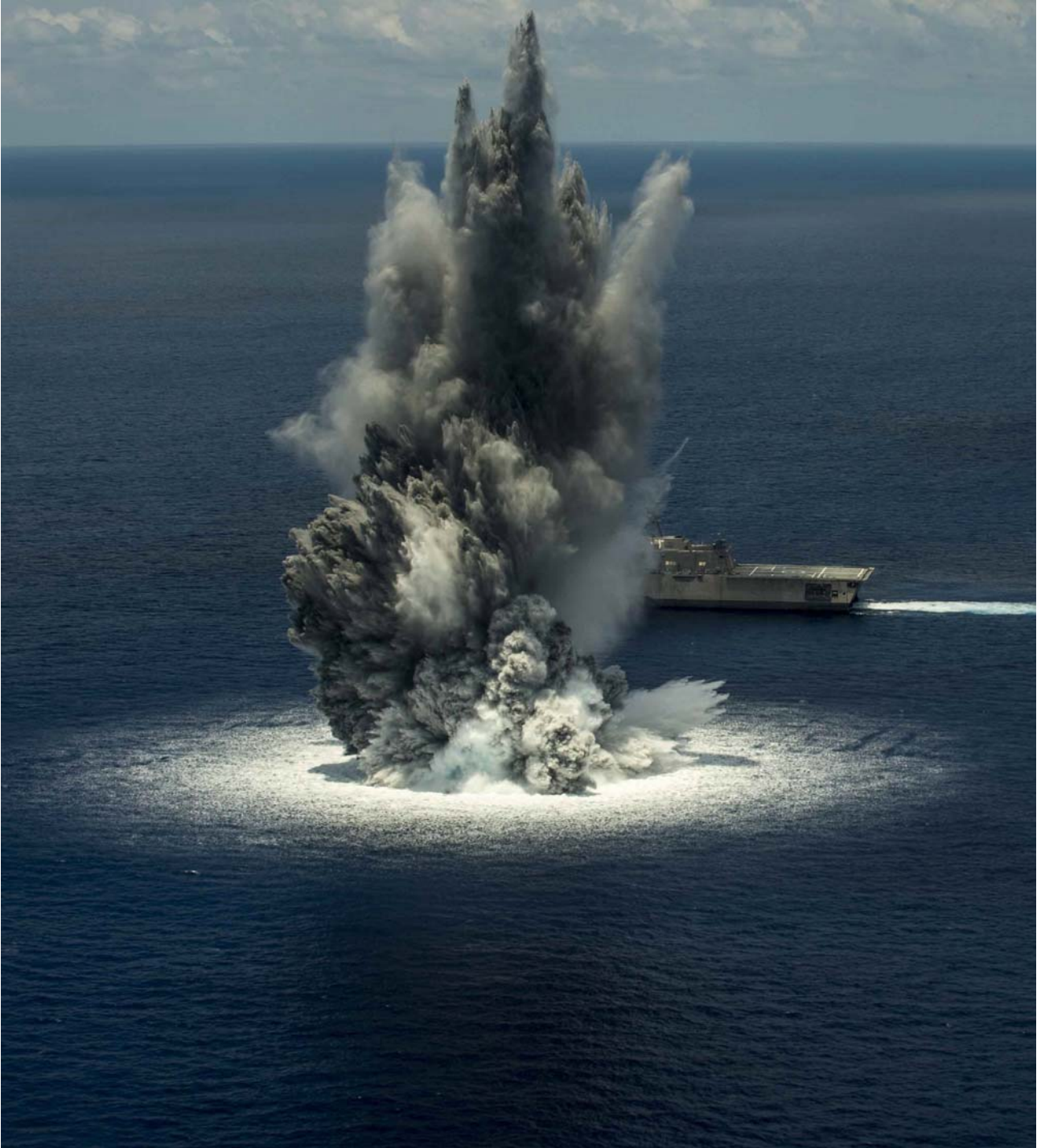
Independence variant Littoral Combat Ship USS Jackson (LCS 6) completing the first of three full-ship shock trials in 2016. (U.S. Navy photo by Mass Communication Specialist 2nd Class Michael Bevan/Released)
