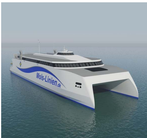
Render of 109 metre vehicle passenger ferry to be constructed for Mols Linien of Denmark, by Austal Australia
