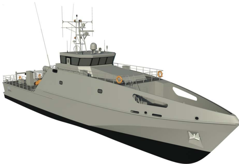
Render of 40 metre Pacific Patrol Boat Replacement (PPB-R) – 19 steel vessels to be constructed by Austal Australia for 12 Pacific Island nations from 2018 - 2023
