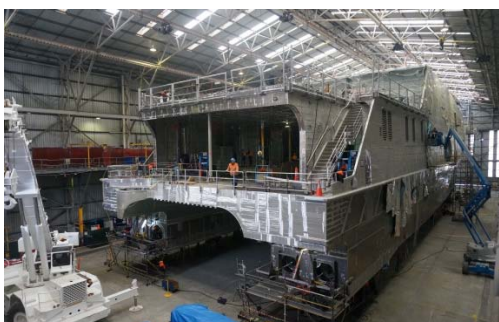
High Speed Support Vessel (HSSV) under construction at Austal Australia
